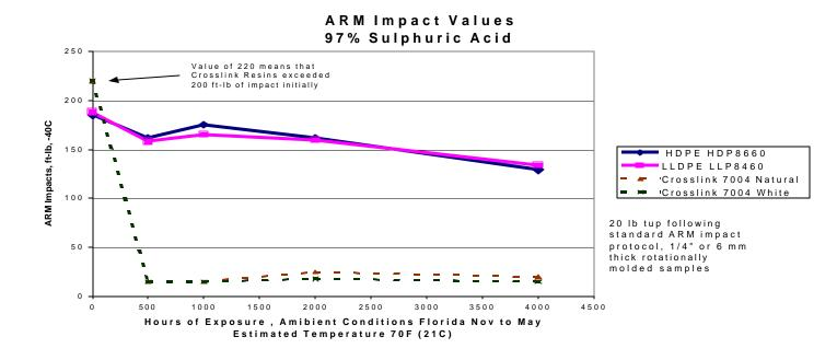
Ductility in ARM Impact Test 97% Sulphuric Acid (Higher Value Represents More Ductility)
