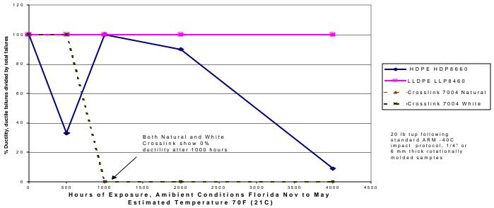
All samples start with good ductility with the crosslink samples having higher impact values than the HDPE or LLDPE. However, the HDPE and LLDPE samples retain more of their initial impact values and ductility after 1000 hours of exposure.
